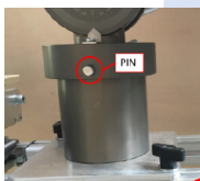
Platform yaw rotation scale 360^\circ (pinhole at every 90^\circ )
