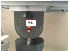
Platform pitch rotation scale, -90^\circ to +90^\circ
